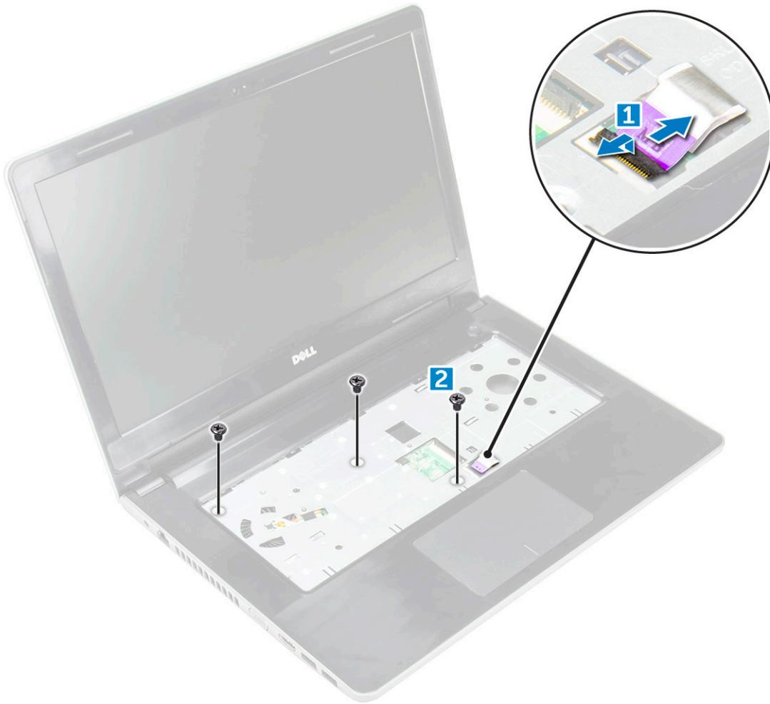
4 Remove the screws that secure the base cover to the computer
