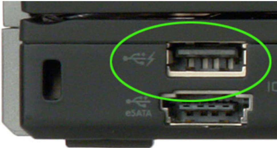
Only the USB connector with a **lightning bolt icon**, as seen in the image above, can be used.
