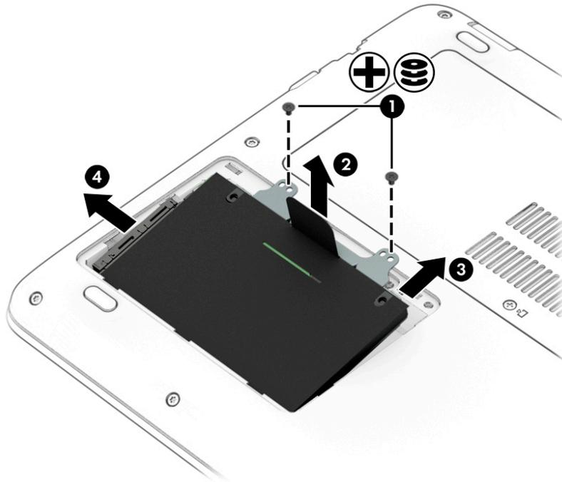
4. To remove the hard drive cover from the hard drive, remove the 4 Phillips PM3.0×3.0 screws (1) that secure the bracket to the drive, and then lift the cover off the drive (2).
