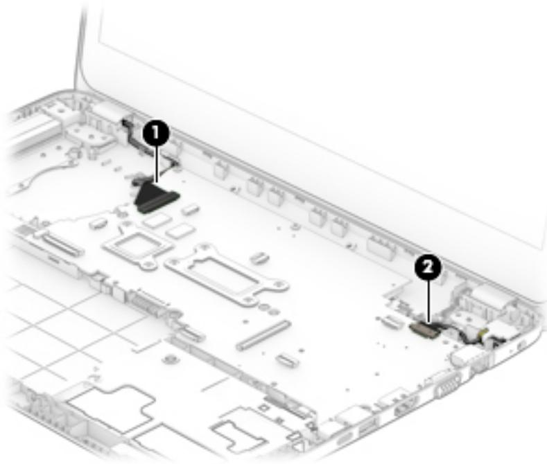
3. Remove the 3 Phillips PM2.5×5.0 screws (1) that secure the system board to the computer.
