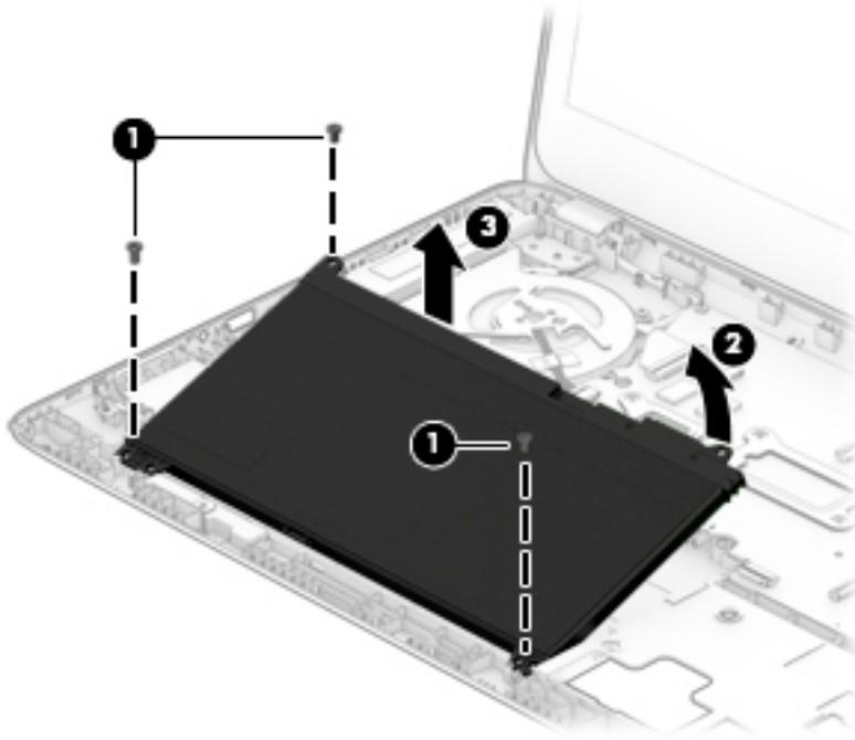
Reverse this procedure to install the battery.
