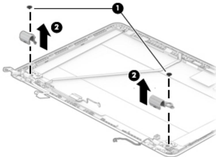
15. If it is necessary to remove or replace the display hinges, remove the 6 Phillips PM2.5×2.5 screws **(1)** that secure both display hinges to the display enclosure.
