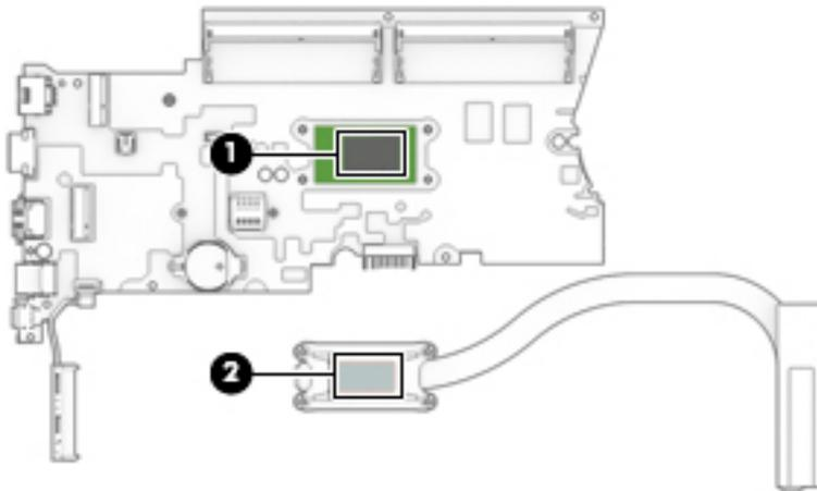
Reverse this procedure to install the heat sink assembly.
