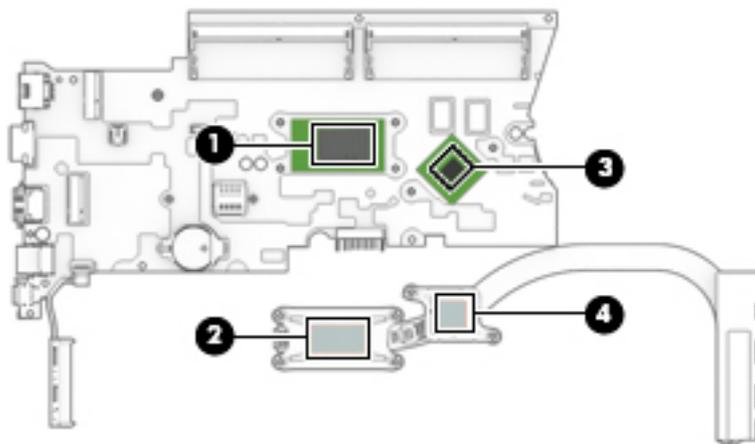
4. **UMA models:** In the order indicated on the heat sink, loosen the 4 captive Phillips screws (1)–(4) that secure the heat sink to the system board.
