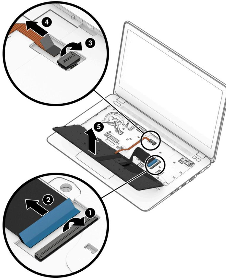
Reverse this procedure to install the keyboard.
