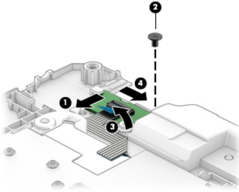
Reverse this procedure to install the function board.
