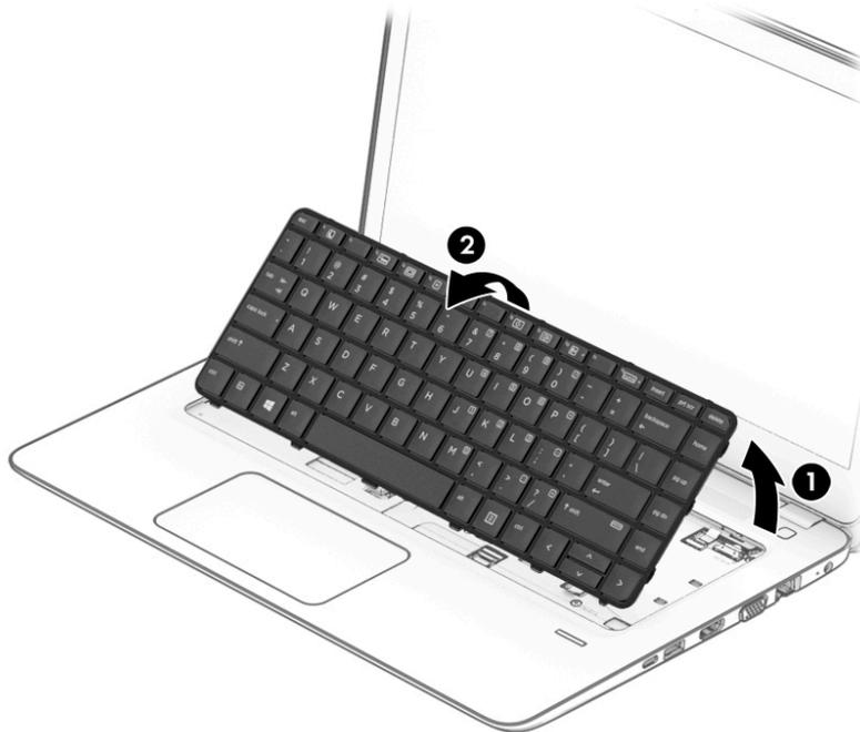
4. Disconnect the keyboard cable by lifting the connector latch (1), and then disconnect the keyboard cable from the system board (2).
