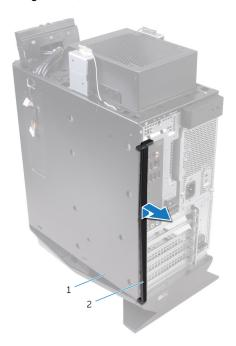
Figure 45. Removing the rear trim cover
