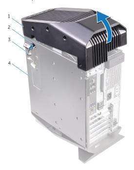
Figure 7. Removing the top cover
