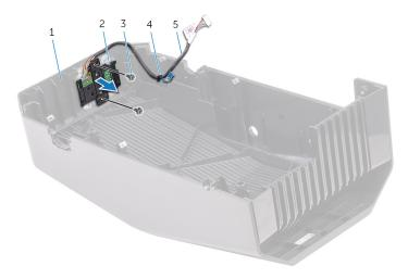
Figure 43. Removing the power-button module
