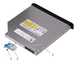
Figure 39. Removing the optical drive
