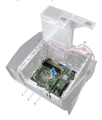
Figure 47. Removing the system board
