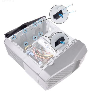
Figure 11. Releasing the bottom cover from the chassis
