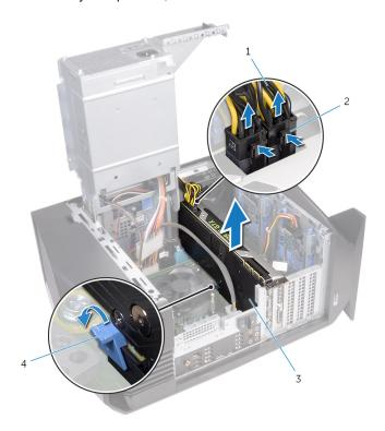
Figure 25. Removing the graphics card
