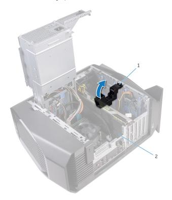
Figure 24. Removing the graphics card
