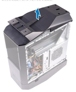
Figure 12. Removing the bottom cover
