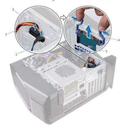
Figure 15. Removing the hard drive
