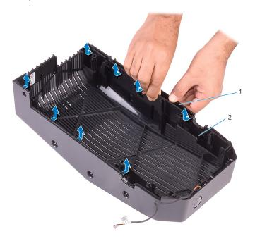
Figure 8. Releasing the top cover from the top bezel
