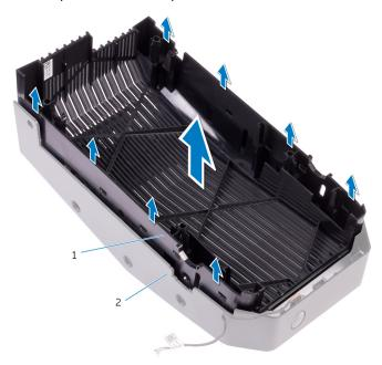
Figure 9. Lifting the top cover from the top bezel
