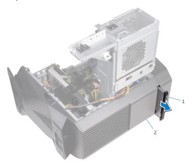
Figure 38. Removing the optical drive
