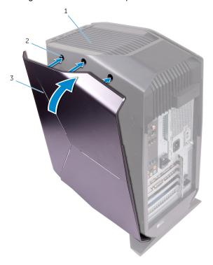
Figure 5. Replacing the right-side cover
