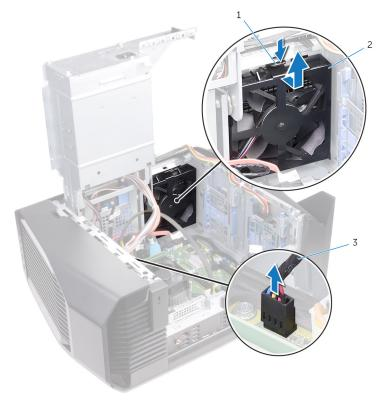
Figure 33. Removing the chassis fan
