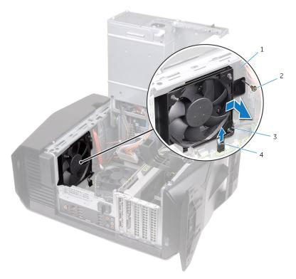
Figure 35. Removing the top-chassis fan
