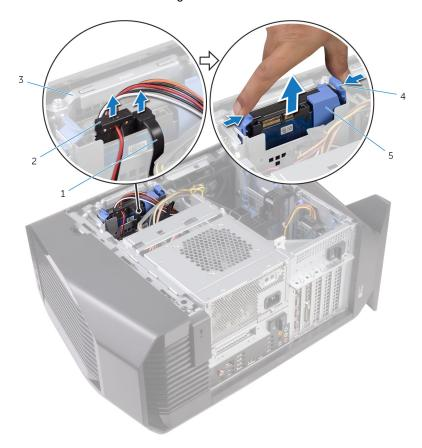
Figure 13. Removing the hard drive
