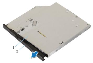
Figure 40. Removing the optical drive
