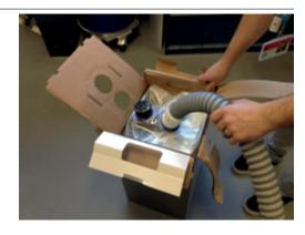
7. Switch-on the explosion-protected vacuum cleaner to remove the air from the bag while pushing it downwards to separate the plastic bag from the cardboard.
