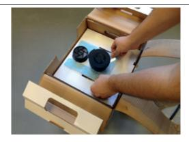
4. Rotate the cartridge connector and remove it carefully to avoid spreading any material left on it.
