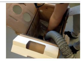
8. Take out the collapsed bag and remove the connector from the explosion-protected vacuum cleaner.
