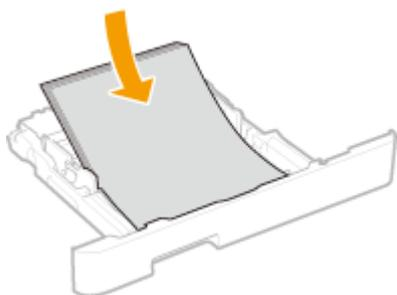
**IMPORTANT:****Do not exceed the load limit line when loading paper**
