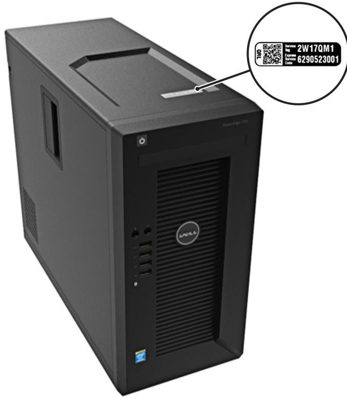
Figure 54. Locating Service Tag of your system
