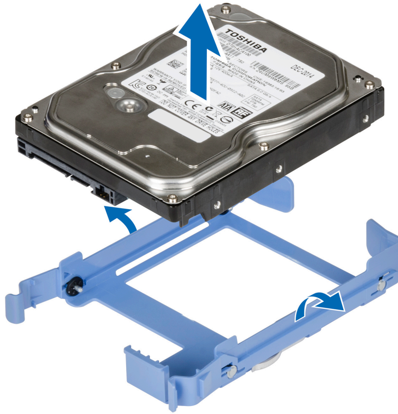
Figure 26. Removing a hard drive from a hard drive carrier
