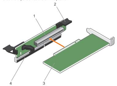
Figure 52. Installing an expansion card
