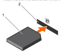
Figure 56. Installing the SD vFlash card
