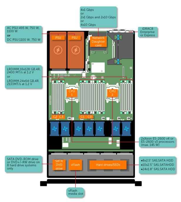
Figure 1. Supported configurations for PowerEdge R630 system
