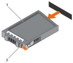
Figure 29. Removing a 2.5-inch hard drive blank
