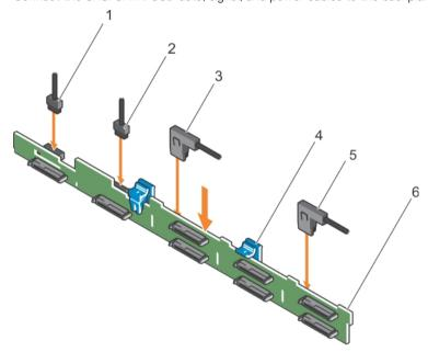
Figure 86. Installing the 2.5-inch (x8) hard drive backplane
