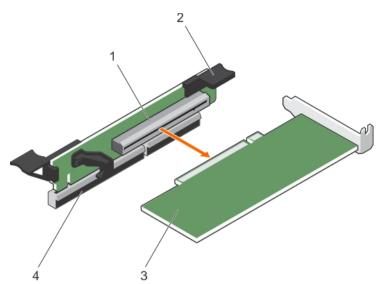
Figure 51. Removing an expansion card
