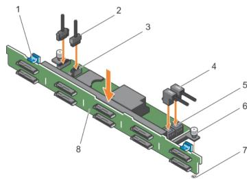
Figure 87. Installing the 2.5-inch (x10) hard drive backplane
