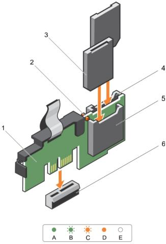
Figure 58. Installing the optional internal dual SD module
