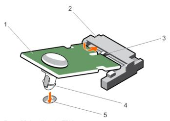
Figure 99. Installing the TPM
