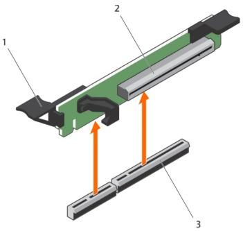
Figure 50. Removing the expansion card riser 3
