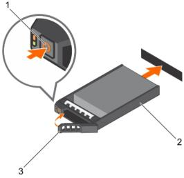
Figure 35. Installing a hot swappable hard drive
