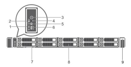
Figure 2. Front panel features of the 10  $\times$  2.5-inch hard drive PowerEdge R630 chassis
