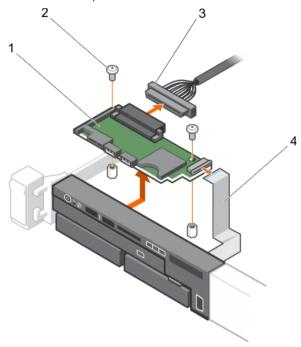
Figure 89. Removing the control panel board
