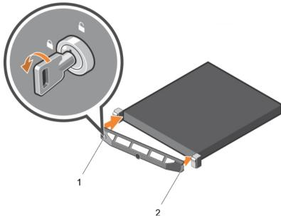
Figure 18. Installing the optional front bezel
