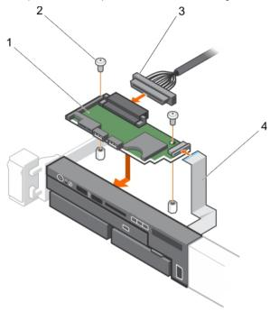
Figure 90. Installing the control panel board
