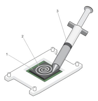
Figure 66. Applying thermal grease on the top of the processor
