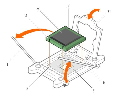
Figure 65. Removing and installing a processor
