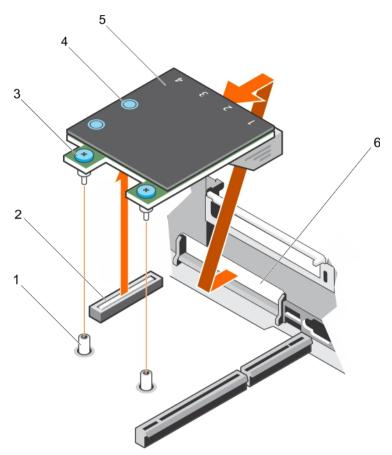
Figure 61. Removing the NDC
