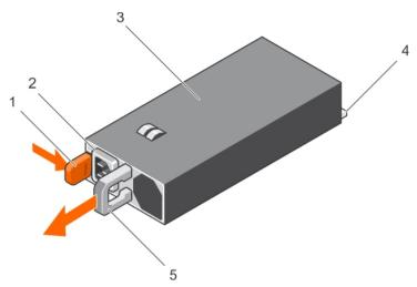
Figure 70. Removing an AC PSU
