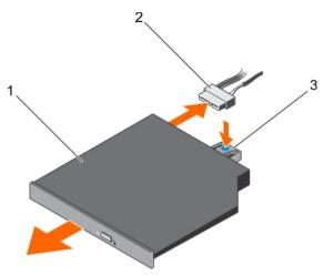
Figure 41. Removing the optional optical drive
