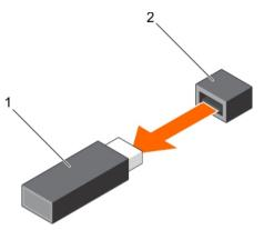
Figure 47. Removing the internal USB memory key
