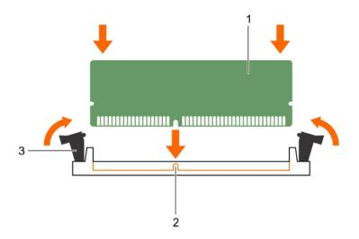
Figure 28. Installing the memory module
