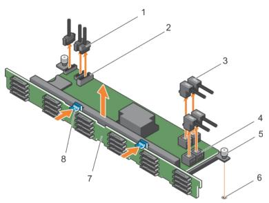
Figure 84. Removing the 1.8-inch (x24) hard drive backplane
