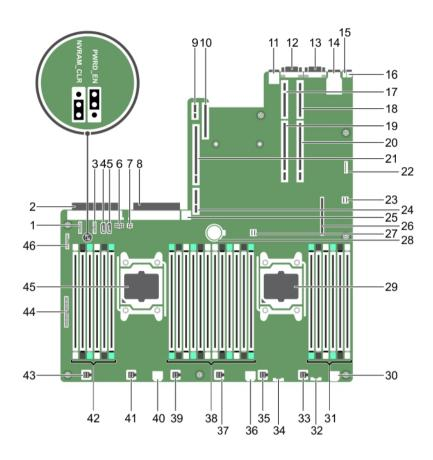
Figure 100. System board jumpers and connectors
