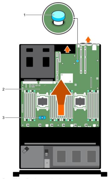
Figure 98. Installing the system board
