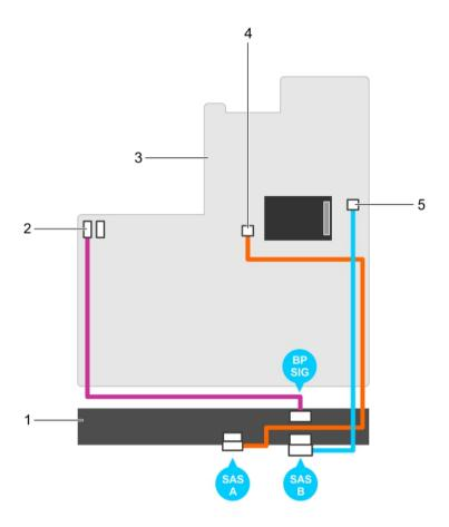
Figure 81. Cabling diagram—2.5-inch (x8) hard drive systems
