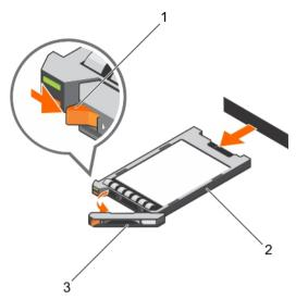
Figure 34. Removing a 1.8 inch hot-swappable uSATA SSD carrier
