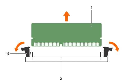
Figure 27. Removing the memory module
