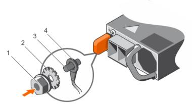
Figure 72. Assembling and connecting the safety ground wire
