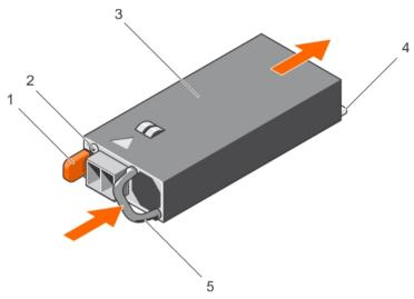
Figure 77. Installing a DC PSU
