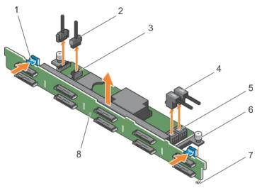
Figure 82. Removing the 2.5-inch (x10) hard drive backplane
