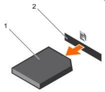
Figure 55. Removing the SD vFlash card
