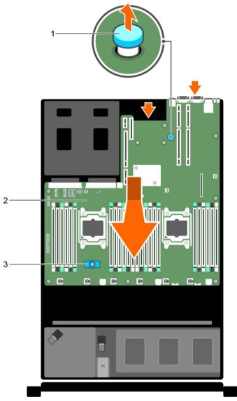
Figure 97. Removing the system board
