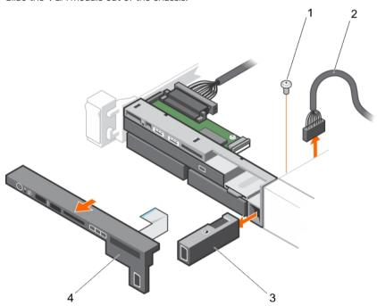
Figure 95. Removing the VGA Module
