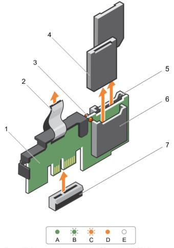
Figure 57. Removing the internal dual SD module (IDSDM)
