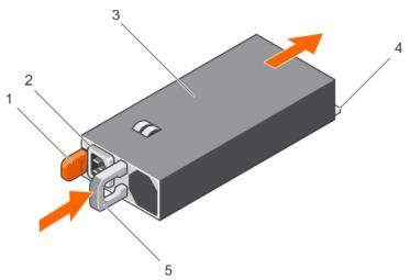
Figure 71. Installing an AC PSU
