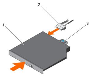
Figure 42. Installing the optional optical drive
