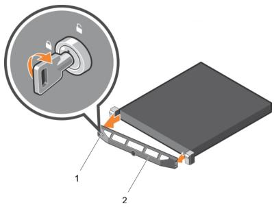
Figure 16. Removing the optional front bezel
