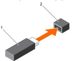
Figure 48. Installing the internal USB memory key
