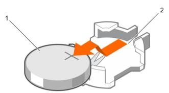
Figure 78. Removing the system battery
