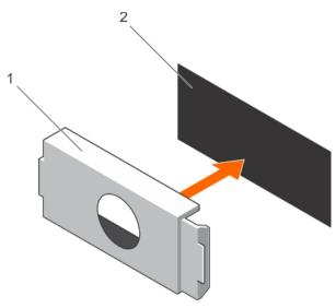
Figure 69. Installing the PSU blank
