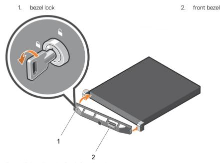
Figure 19. Installing the Quick Sync bezel
