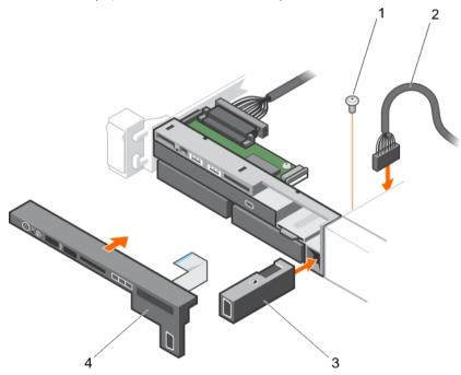
Figure 96. Installing the VGA module
