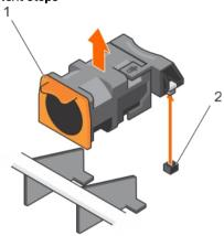
Figure 45. Removing a cooling fan
