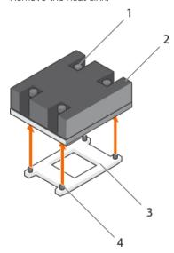
Figure 63. Removing a heat sink
