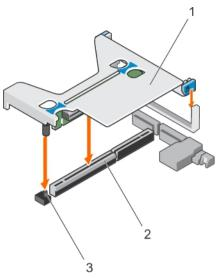
Figure 53. Installing the expansion card riser 1
