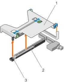
Figure 49. Removing the expansion card riser 1
