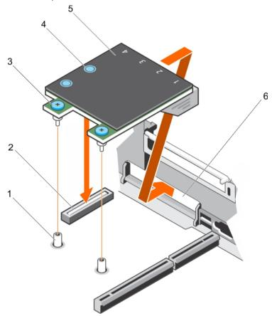
Figure 62. Installing the NDC
