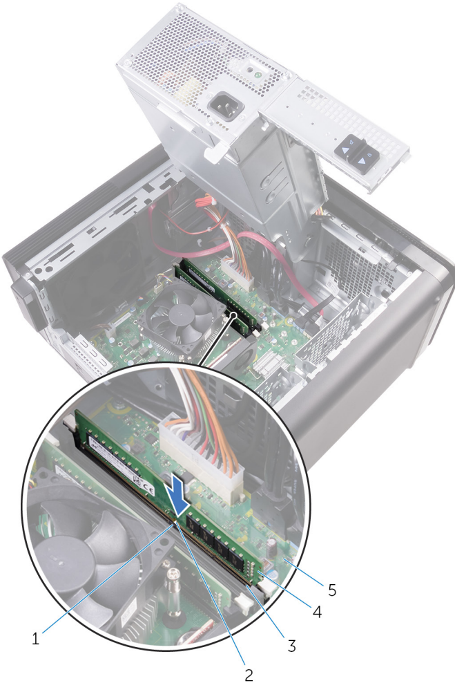
Figure 24. Replacing the memory module
