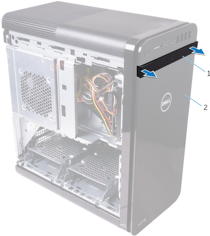
Figure 5. Removing the optical drive bezel
