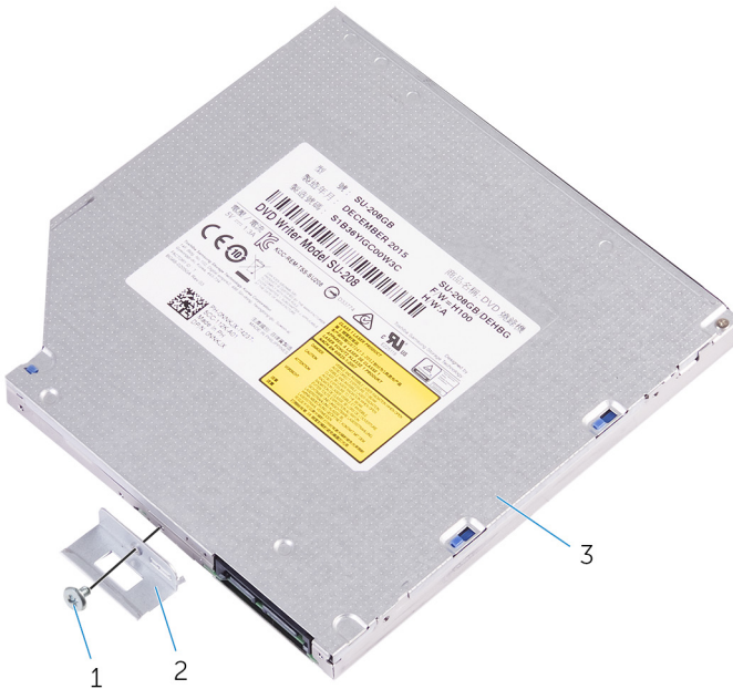
Figure 27. Removing the optical drive
