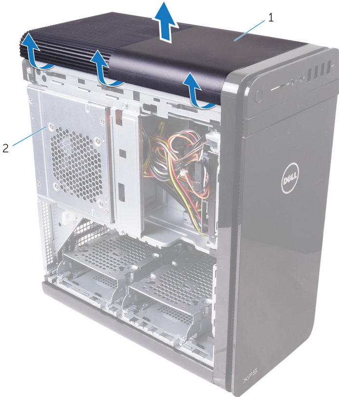
Figure 3. Removing the top cover
