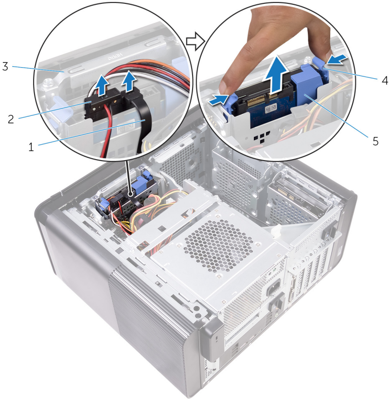
Figure 7. Removing the hard-drive assembly
