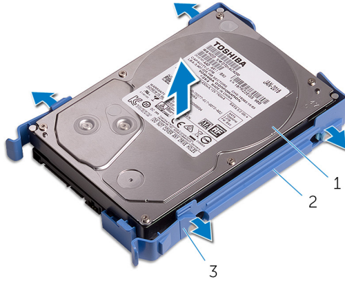
Figure 8. Removing the hard drive from the bracket
