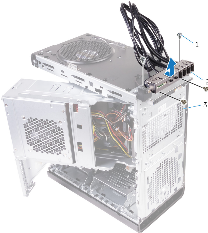
Figure 30. Removing the USB panel
