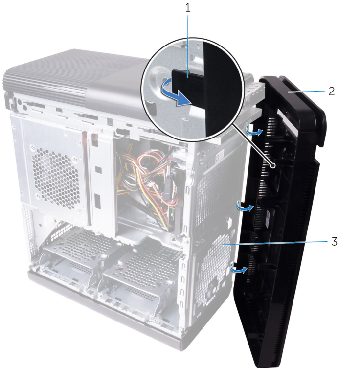
Figure 6. Removing the front bezel
