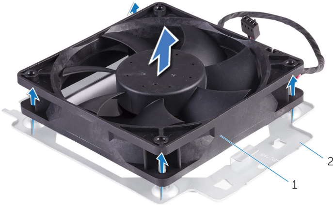
Figure 19. Removing the chassis fan
