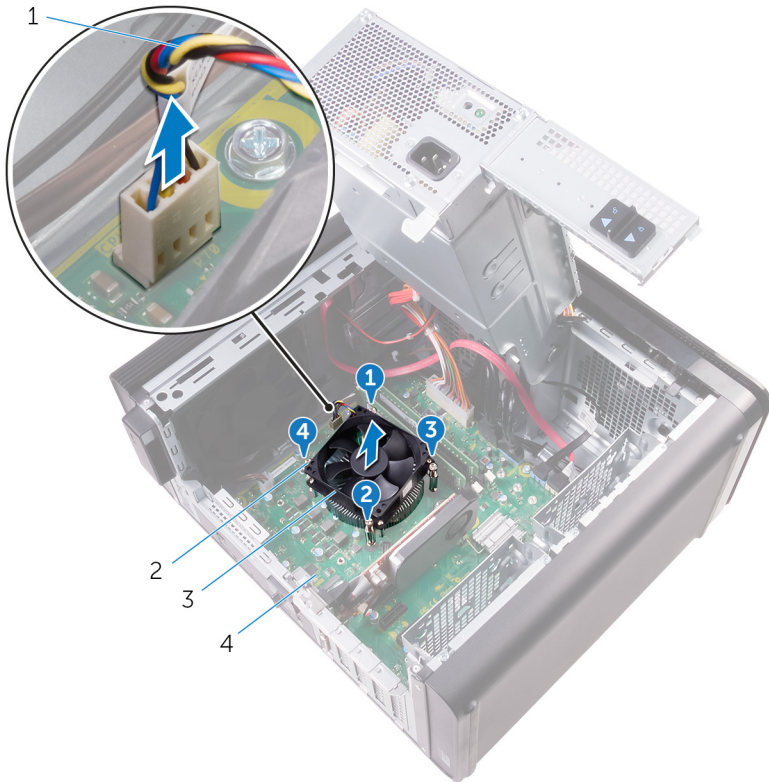
Figure 34. Removing the processor fan and heat sink
