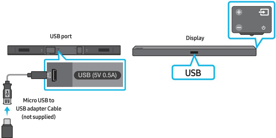
1. Connect a Micro USB to USB adapter cable with a male USB 2.0 Micro USB plug (Type B) on one end and a standard female 2.0 USB jack (Type A) on the other end to the micro USB jack on your Soundbar.
