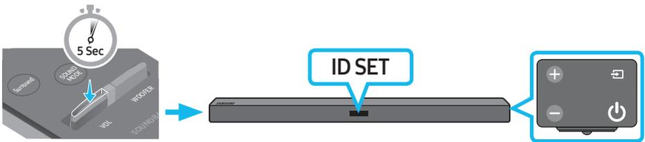
5. When the blue indicator on the subwoofer blinks, turn on the Soundbar's power by pressing **⏻ (Power)** button on the right side of the main unit or on the remote control.
