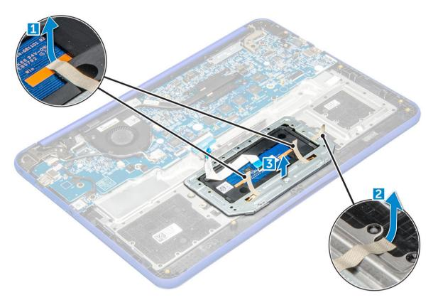
Remove the M2xL3 screws that secure the touchpad to the system [1] and then lift the touchpad from the system [2].
