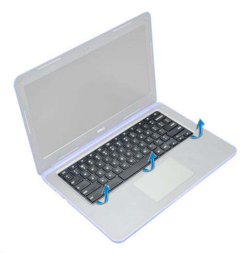
CAUTION: As you remove the keyboard from the palmrest, carefully pull out the keyboard cable from the opening on the palmrest.
