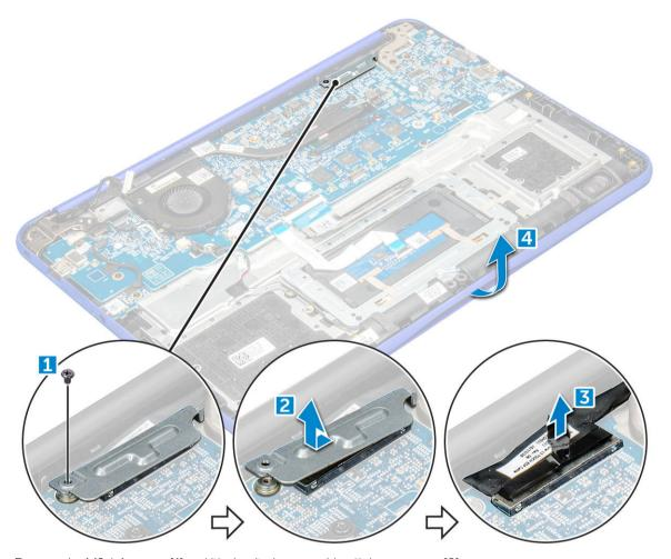
5 Remove the M2xL4 screws [1] and lift the display assembly off the computer [2].
