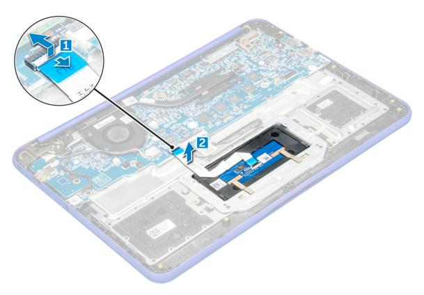
Remove the M2xL3 screws that secure the metal bracket to the touchpad on the computer.
