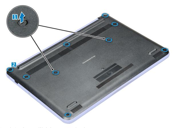
3 Using a plastic scribe, pry and lift the base cover away from the computer.
