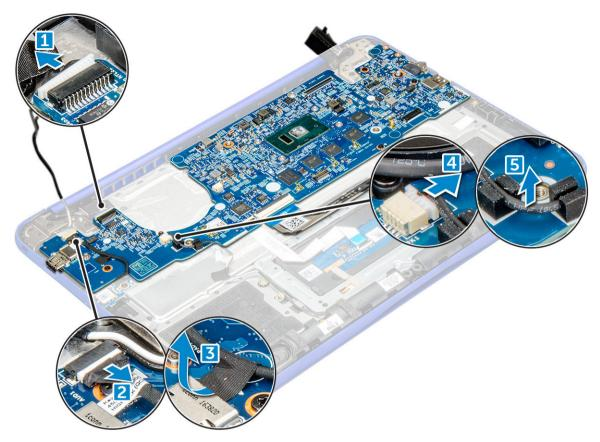
Remove the M2xL3 screws and lift the system board off the computer.
