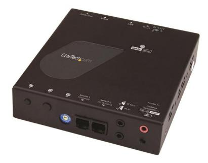
This 4K HDMI® over IP receiver works with the <u>4K HDMI over IP Extender Kit</u> (sold separately) and lets you extend a 4K HDMI signal, as well as RS-232 peripheral device connections, over your network. You can use additional receivers (sold separately) to distribute the HDMI signal to multiple locations, each with 4K support, and combine your remote displays to create a video wall.
