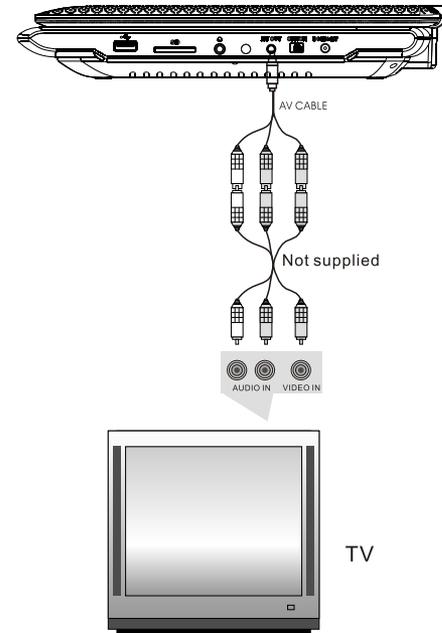
Please use AV cable to connect the machine and the TV. Make sure it is connected correctly.
