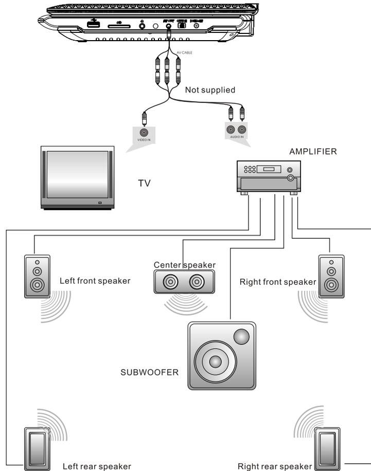
Notice: There is no 5.1 channel in the unit, however, after connecting to APM it is available to output audio in 5.1 channel
