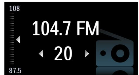
Simply tune into the station that you want to preset, press and hold the preset button to memorize the frequency. With preset radio stations that can be stored, you can quickly access your favorite radio station without having to manually tune the frequencies each time.
