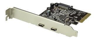
This USB 3.1 card lets you add two USB-C ports to your computer, through a PCI Express slot. It enables you to upgrade your current system by adding two USB 3.1 Gen 2 ports to your computer and giving you access to data transfer speeds up to 10Gbps.
