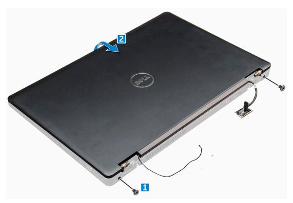
Lift the display assembly away from the computer.
