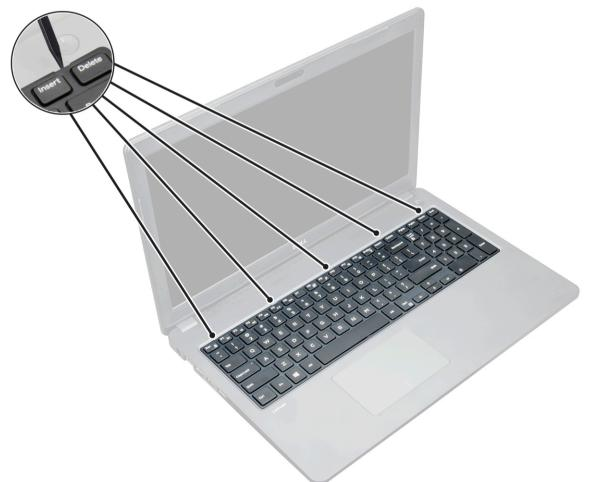
4 Pry out the lower edge of the keyboard [1] and flip it over [2].
