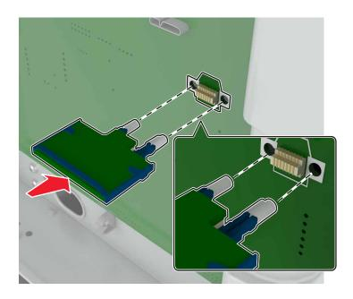
**Note:** The entire length of the connector on the card must touch and be flush against the controller board.
