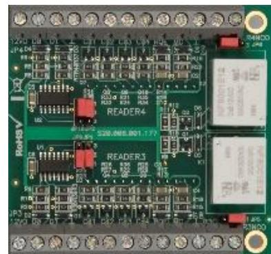
The Asguard ACE plug-in module is used to expand Asguard ACM to 4 readers.
