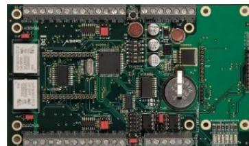
The Asguard ACM can be expanded to 4 readers using the Asguard ACE plug-in module.
