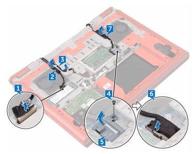
Remove the two screws (M2x3) that secure the display assembly to the computer base.
