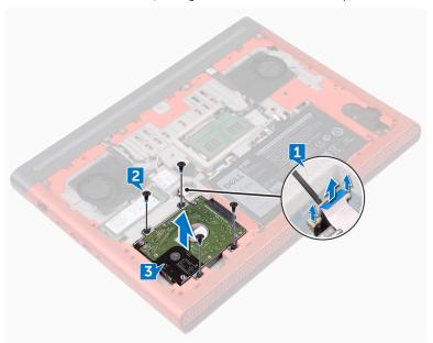
4 Disconnect the interposer from the hard-drive assembly.
