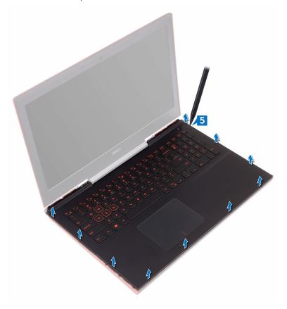
Lift the palm rest and keyboard assembly at an angle.
