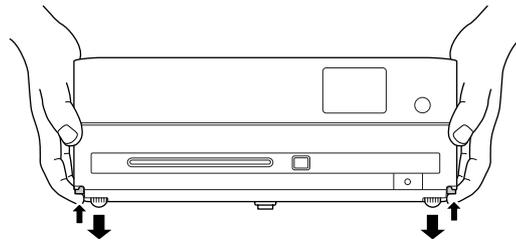
Adjust the front feet by pressing the foot levers. You can tilt the projector up to 10°. Adjust the feet in such a way that the unit is level.
