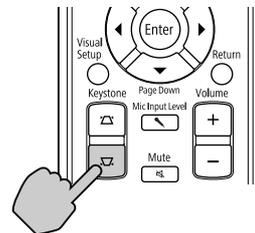
If the unit is tilted by up to 30° degrees in an upward or downward orientation, you can correct the image shape. However, it will be difficult to focus if the tilt angle is large.
