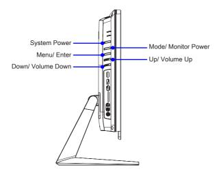
Press the Menu button to launch the OSD main menu. Use the Up and Down buttons
