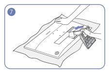
Push the assembled stand into the main body in the direction of the arrow, as shown in the figure.
