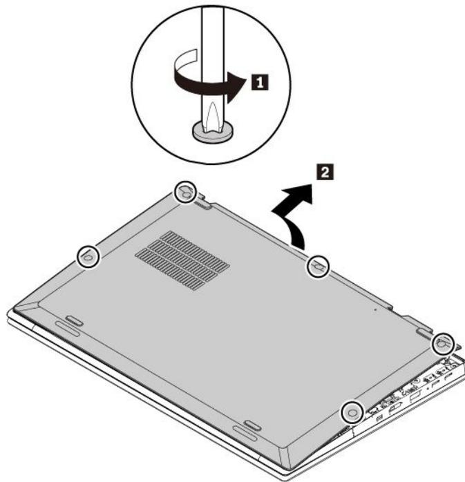
5. Install a new base cover assembly in place **1**. Press the left and right sides of the base cover assembly as shown **2**, and then tighten the screws in ascending alphabetical order (a to e) as illustrated **3**.
