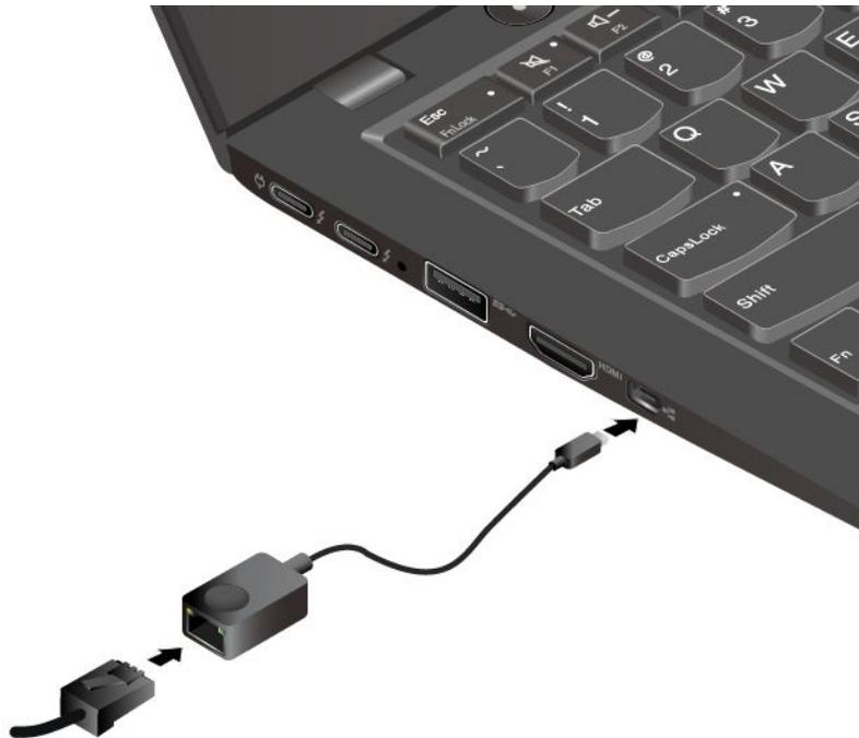
The Ethernet connector has two indicators that show the status of the network connection. When the green indicator is on, the computer is connected to a LAN. When the yellow indicator blinks, data is being transmitted.
