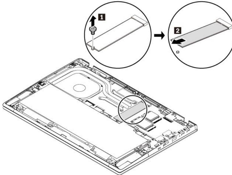
6. Install a new M.2 solid-state drive by doing the following:
