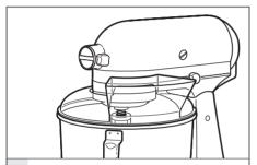
For best results, rotate the shield so the motor head covers the U-shaped gap in the shield. The pouring chute will be just to the right of the attachment hub as you face the Stand Mixer.
