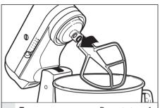
To remove accessory: Repeat steps 1 and 2. Press accessory upward 4 as far as possible and turn to the left. Then pull accessory from the beater shaft.
