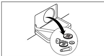
3. Remove any extraneous matter from the pump filter.
