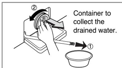
2. Unplug the drain plug. Open the filter by turning to the left.
