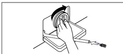
4. After cleaning, turn the pump filter and insert the drain plug.
