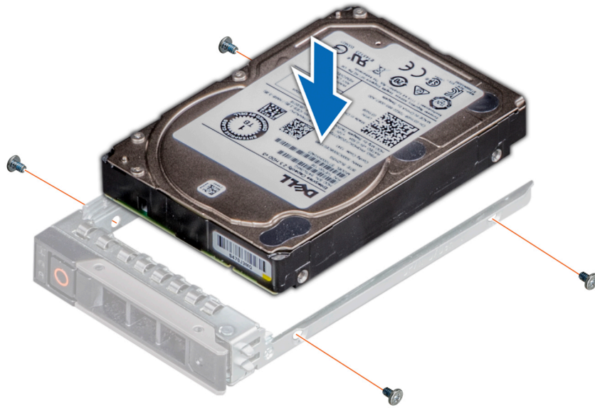
Figure 40. Installing a hard drive into the hard drive carrier
