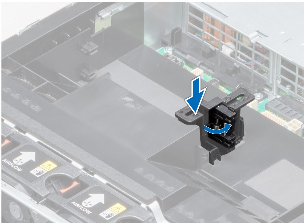
Figure 51. Opening the PCIe card holder latch
