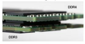
Figure 2. Thickness difference
