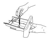
**3.** Clean all parts under running water, removing all detergent or softener residues.
