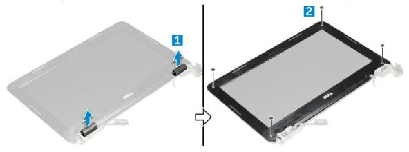
4 Remove the M2.5x3.5 screws and pry the edges to release the display bezel from the display assembly
