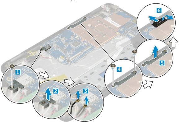
6 Remove the M2. x3.0 screws and lift system board away from the computer[1,2]
