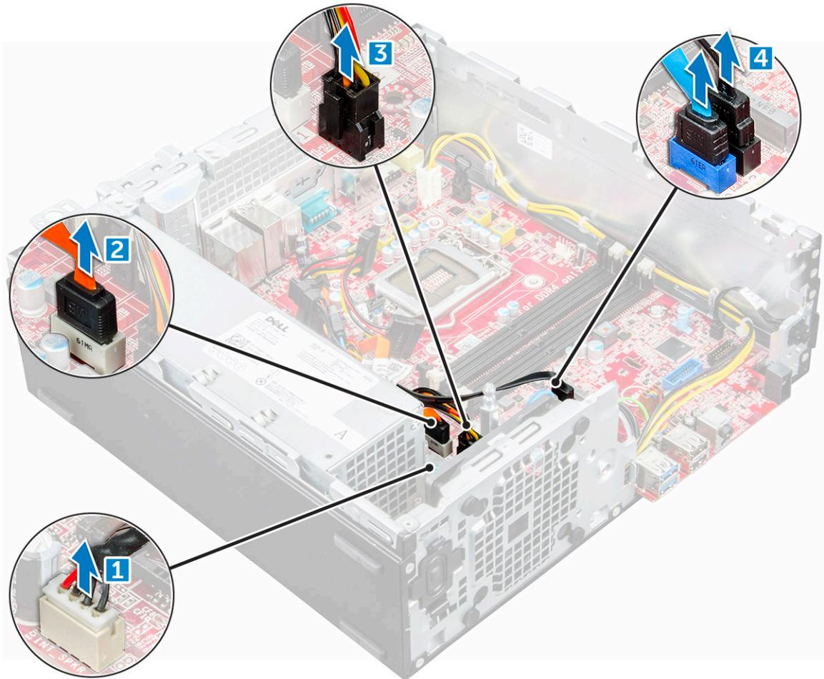
5 Disconnect the following cables and screw from the system board:
