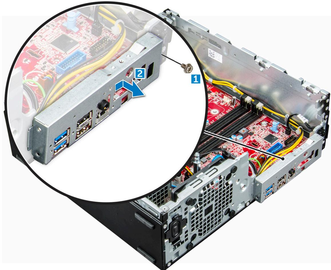
4 Disconnect the following cables from the system board:
