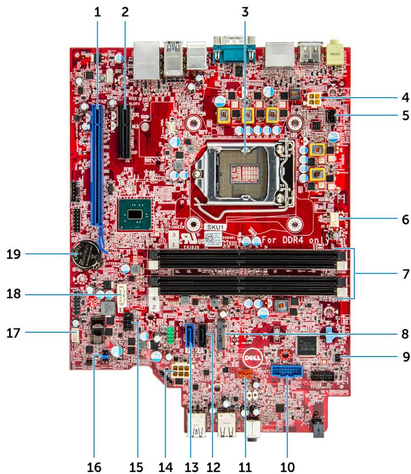
1 PCI-e x16 connector (slot 2)
