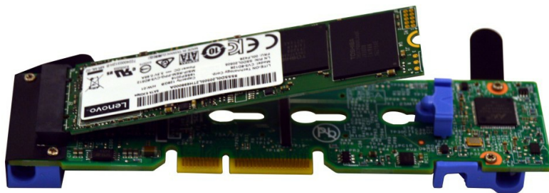
Figure 17. Dual M.2 Boot Adapter and a 128 GB M.2 drive
