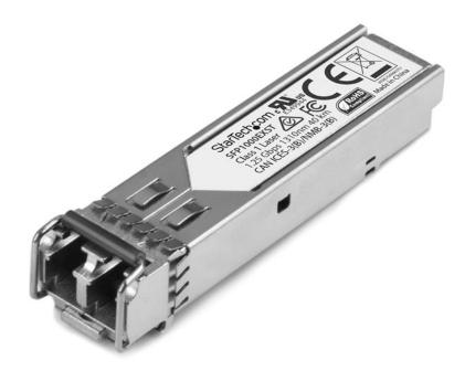
The SFP1000EXST is an MSA compliant fiber SFP transceiver that's designed, programmed and tested to work with 1000BASE-EX compatible MSA switches and routers. The SFP transceiver module supports a maximum distance of up to 40 km (24.8 mi) and delivers dependable 1 GbE connectivity over fiber cabling.
