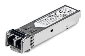
The SFP100BLHST is an MSA compliant fiber SFP transceiver that's designed, programmed and tested to work with 100BASE-LH compatible MSA switches and routers. The SFP transceiver module supports a maximum distance of up to 80 km (49.7 mi) and delivers dependable 100 Mb Ethernet connectivity over fiber cabling. <br/>
