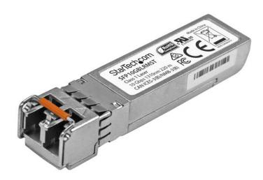
The SFP10GBLRMST is an MSA compliant fiber SFP transceiver that's designed, programmed and tested to work with 10GBASE-LRM compatible MSA switches and routers. The SFP+ transceiver module supports a maximum distance of up to 220 m (721 ft.) and delivers dependable 10 GbE connectivity over fiber cabling.
