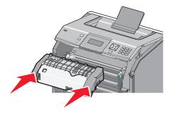
**b** Turn the screws to the right to fasten the fuser unit securely.
