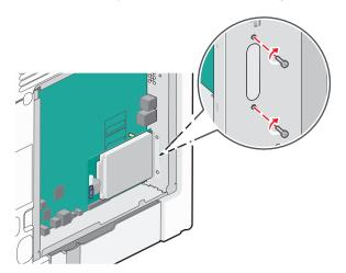
**c** Insert the plug of the printer hard disk interface cable into the receptacle of the system board.
