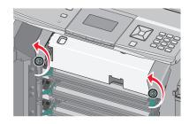
**b** Lift the handholds on each side of the fuser unit, and then pull forward to remove it.
