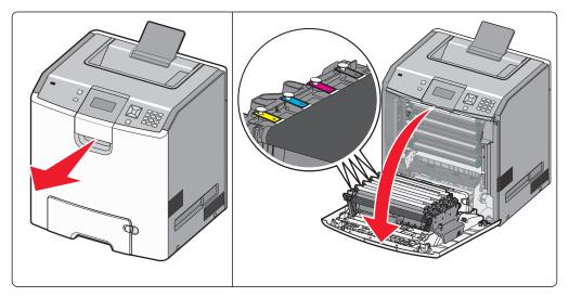
**Warning—Potential Damage:** To avoid overexposing the photoconductors , do not leave the door open for more than 10 minutes.
