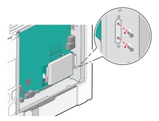
**c** Remove the printer hard disk by pulling it upward to unseat the standoffs.
