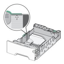
**3** Squeeze the length guide tabs together, and then slide the length guide to the correct position for the size of paper being loaded.
