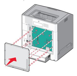
**2** Slide the cover down, and then turn each screw clockwise to tighten.
