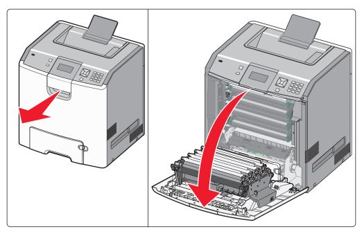
2 Pull up and out on the green tabs of the specified cartridge to remove it from the printer.
