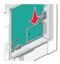
Note: If an optional ISP is currently installed, then the printer hard disk must be installed onto the ISP.
