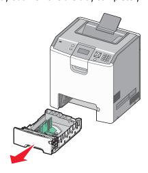
Notice the size indicators on the bottom of the tray. Use these indicators to help position the guides.
