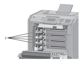
4 Clean the lenses using a can of compressed air.
