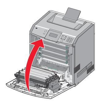
8 If you see 84 Replace <color> photoconductor, 84 <color> photoconductor nearly low, or 84 <color> photoconductor low on the display, then press the up or down arrow button until ✓ Supply Replaced appears, and then press ✓.
