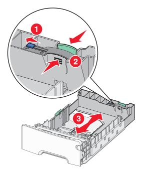
**Note:** The length guide has a locking device. To unlock the tray, slide the button on top of the length guide to the left as shown. To lock the tray once a length has been selected, slide the button back to the right.
