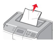
**2** If the jam is under the rollers near the fuser:
