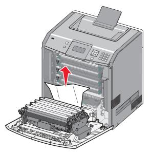
**d** Pull out on the release tabs to allow the front door to split.
