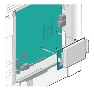
**b** Attach the two provided screws to secure the printer hard disk mounting bracket.
