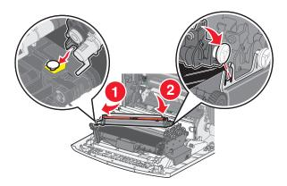
**5** Remove the red packing strip from the top of the photoconductor.
