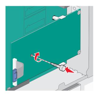
**9** Attach the two provided screws to secure the ISP mounting bracket to the system board cage.
