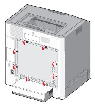
**b** Slide the cover up until each screw is in the keyhole.
