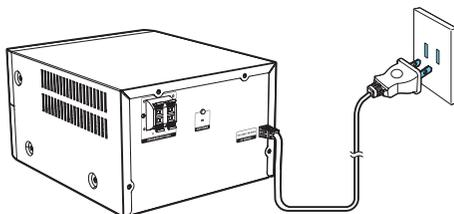
Connect the power cable to the wall socket.
