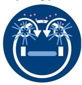
First two long brushes swipe dirt and dust into the path of the robot. Then, the nozzle picks up dirt and dust thanks to its powerful motor. Lastly, the click-on mopping pad enhances the cleaning by collecting even the finest dust from your floors.
