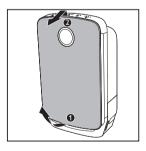
To remove the pre-filter, press the two clips down and pull the filter towards you.
