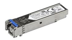
The SFP100BBXUST is an MSA compliant upstream fiber SFP transceiver which pairs with StarTech.com's SFP100BBXDST. They are designed, programmed and tested to work with 100BASE-BX compatible MSA switches and routers. The SFP transceiver module supports a maximum distance of up to 10 km (6.2 mi) and delivers dependable 100 Mbps connectivity over fiber cabling.
