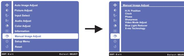
An adjustment page appears after you press the SELECT Button. Then, select V. Position by using the ◀ / ▶ Buttons. Press the SELECT Button again. Then, use the ◀ / ▶ Buttons to change the vertical position settings. The vertical position of the overall display should be changing accordingly while you are doing this.
