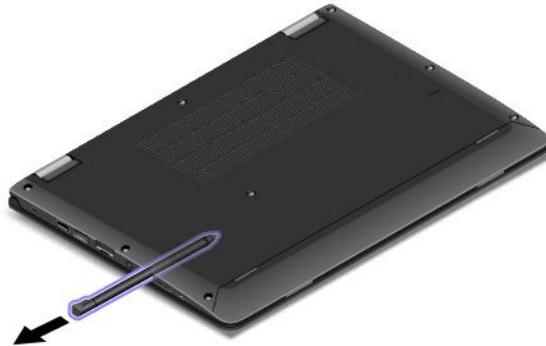
To charge the pen, insert the pen slightly into the slot until it snaps into position. The pen will be fully charged in about five minutes.
