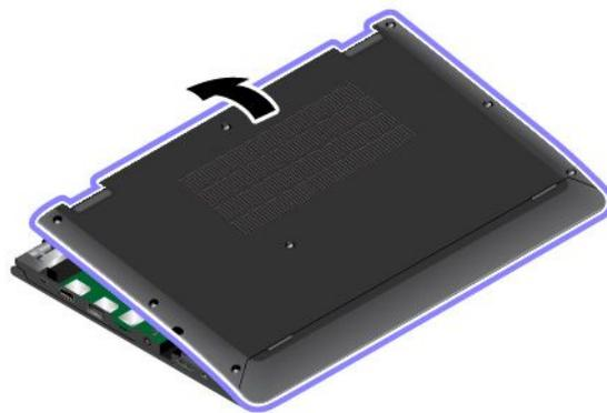
7. Tighten the screws to secure the base cover assembly.
