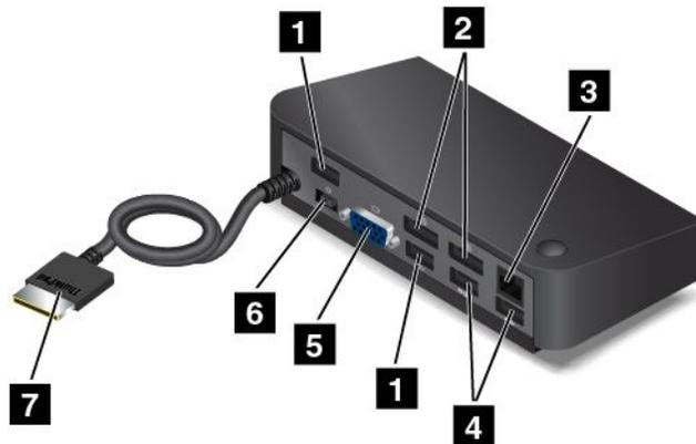
**1 USB 2.0 connectors:** Used to connect devices that are compatible with USB 2.0.
