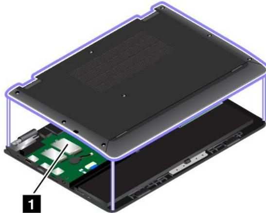
**Note:** For the user-replaceable wireless module, ensure that you use only Lenovo-authorized wireless modules for the computer. Otherwise, an error message will be displayed and the computer will beep when you turn on the computer.
