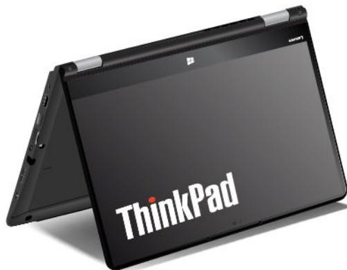
In the tent mode, the keyboard, the trackpad, and the TrackPoint pointing stick are automatically disabled. However, you can control some functions of your computer through the special buttons and the multi-touch screen. For more information, refer to “Using the tablet buttons” on page 19 and “Using the multi-touch screen” on page 19.
