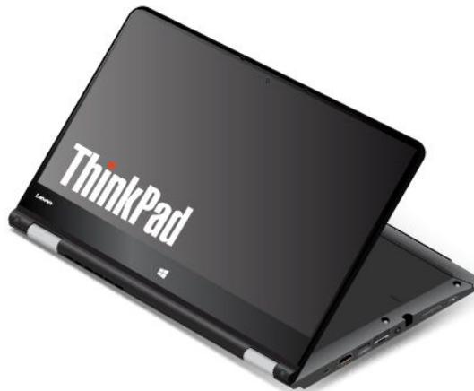
In the stand mode, the keyboard, the trackpad, and the TrackPoint pointing stick are automatically disabled. However, you can control some functions of your computer through the special buttons and the multi-touch screen. For more information, refer to “Using the tablet buttons” on page 19 and “Using the multi-touch screen” on page 19.
