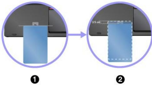
Before you start, ensure that the card is in NFC Data Exchange Format (NDEF), otherwise the card cannot be detected. Then do the following:
