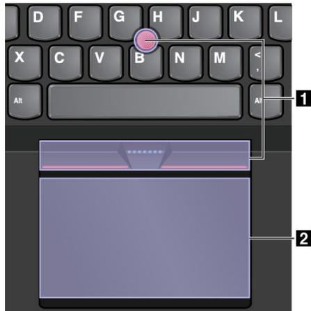
By default, both the TrackPoint pointing device and the trackpad are active with the touch gestures enabled. To change the settings, see “Customizing the ThinkPad pointing device” on page 35.
