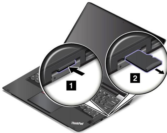
**Installing a micro SD card**
