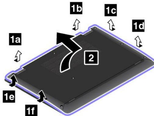
6. Install the new base cover assembly in place.
