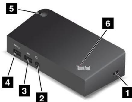
**1 Security-lock slot:** To protect your dock from theft, purchase a security cable lock that fits this security-lock slot to lock your dock to a stationary object.
