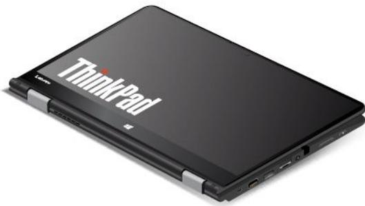
In the tablet mode, the keyboard, the trackpad, and the TrackPoint pointing stick are automatically disabled. However, you can control some functions of your computer through the special buttons and the multi-touch screen. For more information, refer to “Using the tablet buttons” on page 19 and “Using the multi-touch screen” on page 19.
