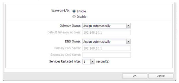
Wake-on-LAN is now enabled. As long as the TeraStation is connected to a power source and the network, you can turn it on remotely.
