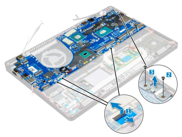
Remove the M2.0x3.0 screws and lift the system board away from the computer [1, 2].
