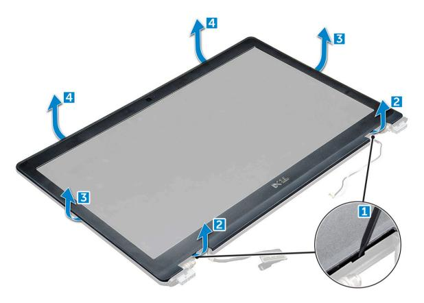
CAUTION: There is a very strong adhesive on the back of the bezel that seals it to the LCD, this can take some force to pry apart from the LCD, care needs to be taken when removing the bezel that the LCD is not damaged
