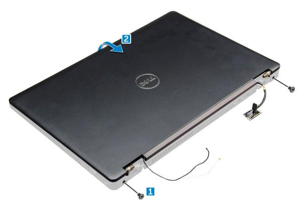
7 Lift the display assembly away from the computer.
