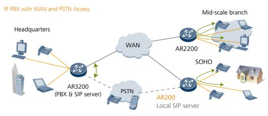
This illustration shows AR200 series router deployed at an enterprise branch with access to a WAN and a PSTN. If a fault occurs on the WAN, the PSTN acts as a backup to the WAN and ensures that call services remain uninterrupted.AR200s are deployed at enterprise branch offices to provide intelligent, integrated dialing across the network. When deployed as voice service gateways, AR200s can function as IP PBX boxes and SIP access gateways.
