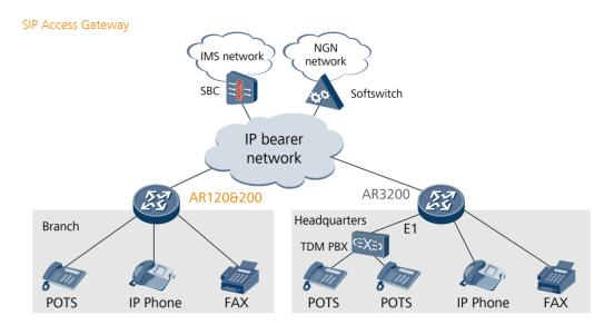
The AR120 and AR200 series routers provide integrated voice, fax, and IP services. The AR120s and AR200s can function as SIP access gateways for enterprise branch offices that transform traditional phone signals into Voice over IP (VoIP). Typically, AR120s and AR200s are connected upstream from the IMS and NGN networks to enable anytime voice communication on any media, such as phones, handsets, and computers.
