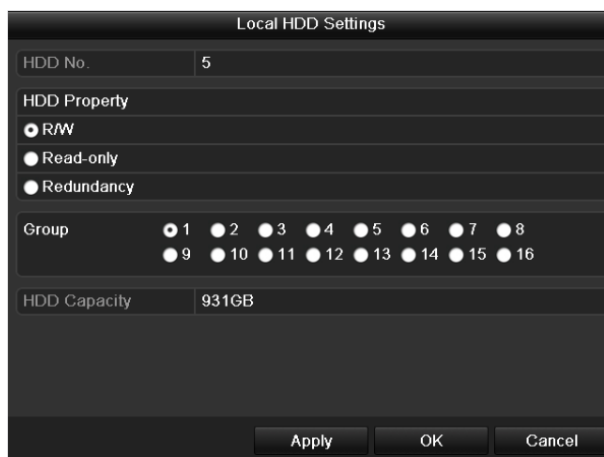
Figure 12. 13 Local HDD Settings Interface
