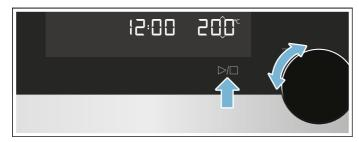
The appliance will start heating. The  $\triangleright/\square$  LED will be lit. The length of the bar on the temperature indicator gradually increases.
