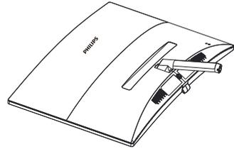
2. Hold the base stand with both hands and firmly insert the base stand into the base column.
