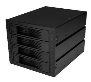
This 4-bay 3.5" SATA/SAS backplane, installed into three standard 5.25" front drive bays, makes it easy to swap 3.5" SATA or SAS drives in and out of your server or desktop computer. It features a trayless design that saves you installation time and enables you to insert or remove drives as needed. With its durable plastic and aluminum construction, it provides a cost-effective solution for drive maintenance and interchangeability of data between multiple systems.
