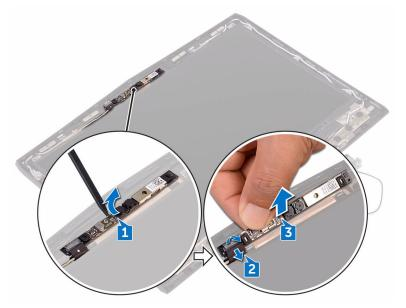
4 Follow the procedure in step 2 in <u>Removing the display back-cover and antenna assembly</u> to remove the camera cable.
