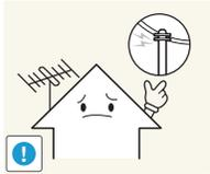
When using an outdoor antenna, be sure to install the antenna away from nearby power lines to prevent the antenna from collapsing onto them in strong winds.
