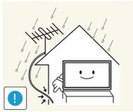
Bend and keep part of the outdoor TV antenna cable hanging downwards (the part inside the room) to prevent rainwater from entering the product.
